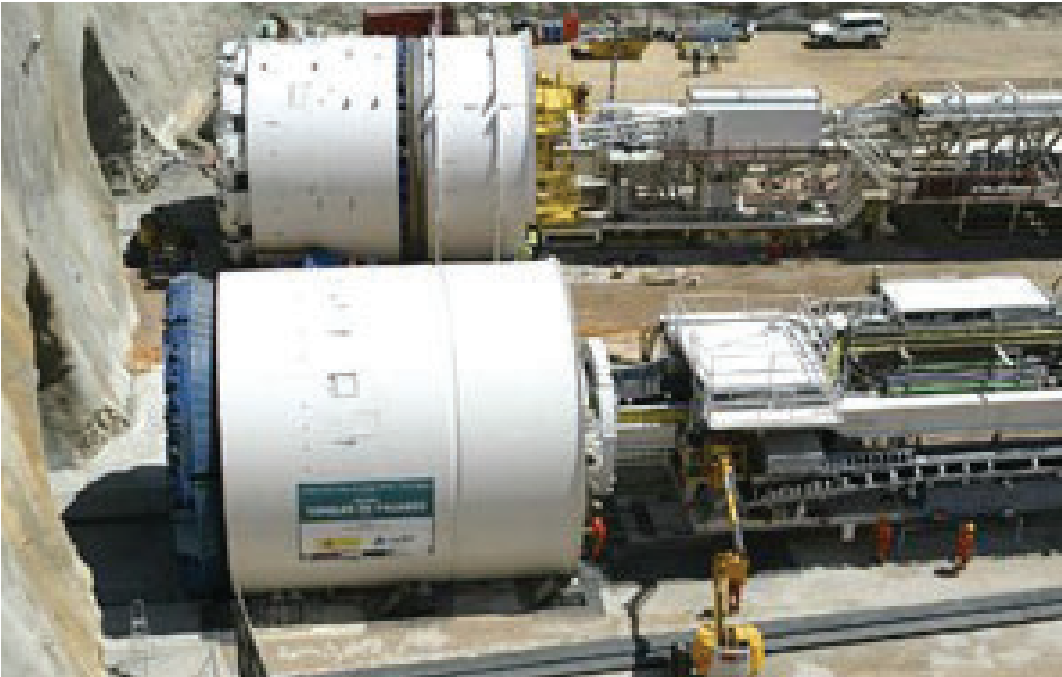
Figure 3. Tunnel boring machines constructing a dual-bore tunnel.
